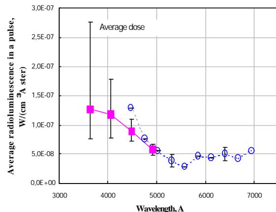
Fig.6. RL spectrum of KU-1 glass under irradiation in the pulse nuclear reactor. Different signs refers to different measurement cycles [12].
