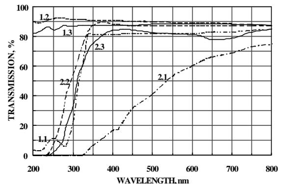
*Fig.1. Optical transmission spectra of sapphire (curves 1.1 and 2.1), quartz glass KU-1 (1.2 and 2.2) and glass KUVI-S (1.3 and 2.3) before (1.1, 1.2 and 1.3) and after (2.1, 2.2 and 2.3) irradiation to nuclear reactor neutron fluence of  $10^{18}$  n/cm<sup>2</sup> and g-dose of 45 MGy [2].*
