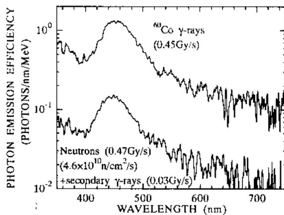
Fig.5. Spectra of photons emitted from high-purity  $\text{SiO}_2$  in DT-neutron and  $^{60}\text{Co}$  gamma ray irradiation experiments at room temperature [9,10]
