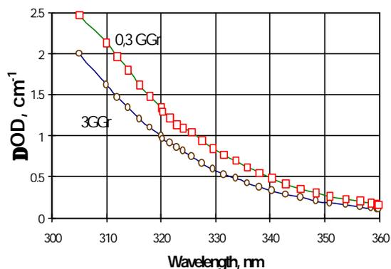
Fig. 2. Radiation induced optical spectra in the short wavelength region after irradiation to different total ionization doses [4].
