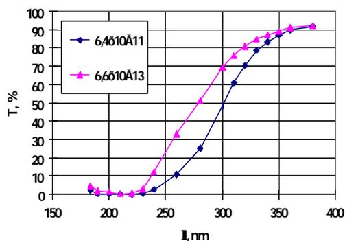
Fig.3 Optical spectra in the UV region for two samples KU-1 with thickness of 2 mm [8]. The values of the neutron flux under irradiation are given in frame in units of  $[n/cm^2 \cdot c]$ .
