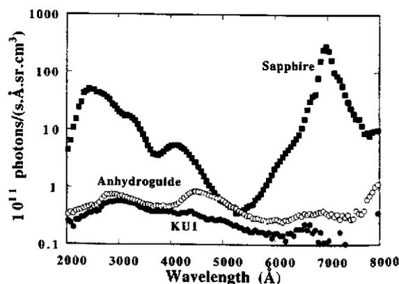
Fig.4. RL spectra for two types of SiO<sub>2</sub> and Union Carbide UV grade sapphire after 2 h irradiation with electrons at 15°C, 700 Gy/s, and  $\sim 10^{10}$  dpa/s [11]
