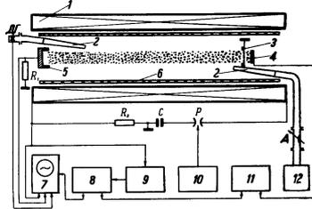
**Fig. 9.** Measuring device: 1—pulse solenoid; 2—dielectric antennae; 3—anode; 4—cathode; 5—collector; 6—chamber; 7—oscilloscope; 8–10—starting device; 11—shaper; 12—8-mm generator
