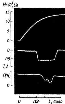
**Fig. 10.** Oscillograms: magnetic field (top); electron beam current (middle); microwave energy passing through the plasma (bottom)
