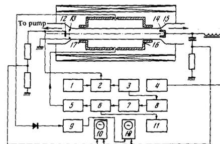
**Fig. 1.** Experimental scheme. 1–15-kV rectifier; 2–pulse-shaping line; 3–trigger; 5–10-db attenuator; 6–power divider; 7–10-cm klystron oscillator; 8–delay line; 9–amplifier; 10–dual-beam oscillographs; 11–frequency meter; 12–cathode; 13–anode; 14–collector; 15–quartz tube; 16–resonator; 17–cutoff waveguides
