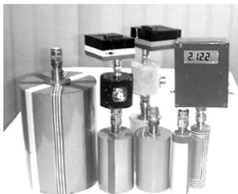
*Fig.1. Different detectors of the neutron registration systems. The size of containers with moderator: cylinders with diameter 3.5, 6.5, and 14 cm and length 12, 11, and 20 cm correspondingly*
