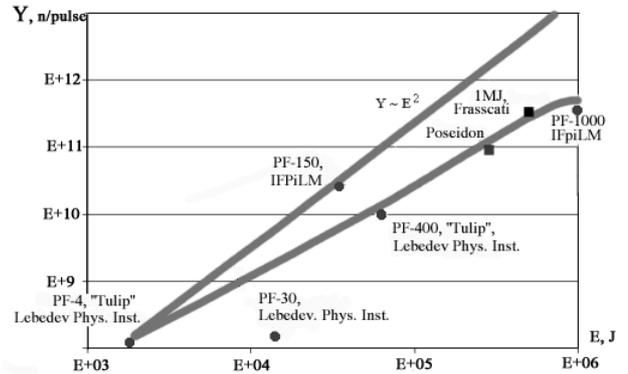
Fig.2. The maximum neutron yield on the different Plasma Focus installations. ●—measurements with these diagnostic systems; ■—data from the literature
