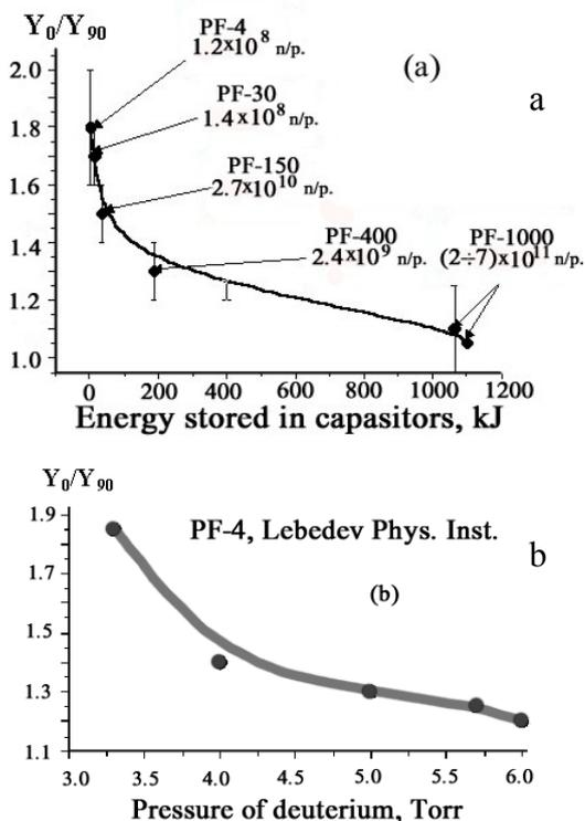
Fig. 3. Spatial neutron anisotropy measured with these neutron activation counters systems
