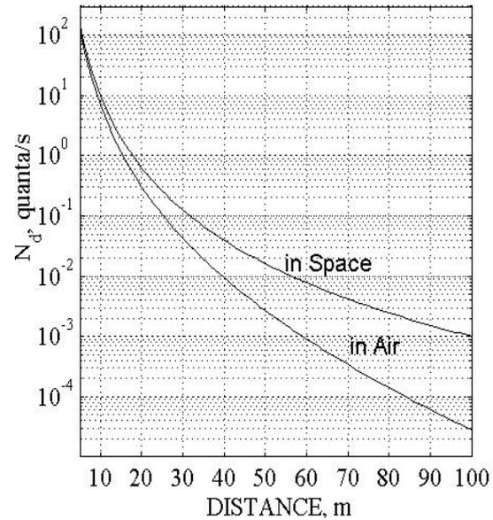
Fig. 2. The number of characteristic radiation quanta (the sum of secondary radiations from all  $K$ -series spectral lines) arriving in 1 sec at the 100  $\text{cm}^2$  detector versus the distance of the locator to the object under inspection. The target irradiated area is 1  $\text{cm}^2$
