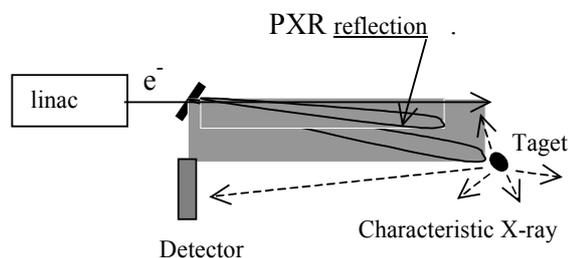
*Fig. 1. General scheme of the monochromatic X-ray locator using the PXR effect. The electron beam from a linac excites PXR in a crystal. Quasi-monochromatic X-ray beam of PXR excites characteristic X-ray radiation in the target (object under inspection). The characteristic X-ray radiation of the target can be registered by a spectrometric detector*
