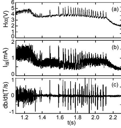
Fig.5. (a)  $H\alpha$ , (b)  $I_{is}$  and (c)  $db/dt$  during H-mode-like phase
