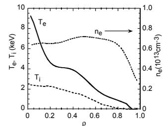
Fig.7. Experimentally obtained  $T_e$  (solid line) and  $n_e$  (dotted line) profiles. Dashed line shows  $T_i$  calculated with neo-classical  $\nu$
