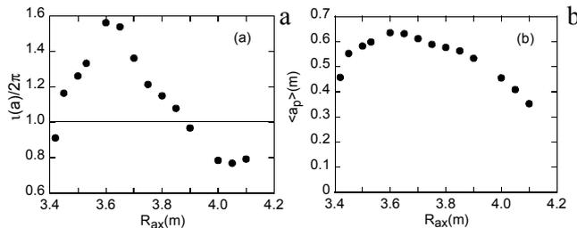
Fig.2. Edge rotational transform (a) and averaged plasma radius (b) against magnetic axis,  $R_{ax}$
