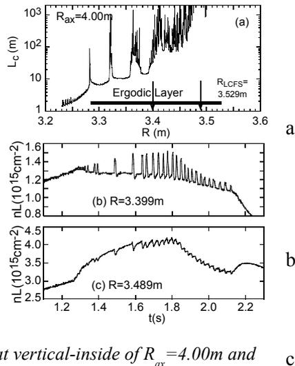
Fig.6. (a)  $L_c$  at vertical-inside of  $R_{ax}=4.00\text{m}$  and (b) (c)  $nL$ . Two arrows indicate positions of 100m.
