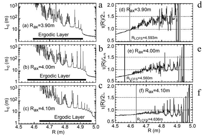
Fig.3. Edge profiles of magnetic field connection length ((a), (b), (c)) and rotational transform ((d), (e), (f)) at  $R_{ax}=3.90\text{m}, 4.0\text{m}$  and  $4.1\text{m}$ , respectively
