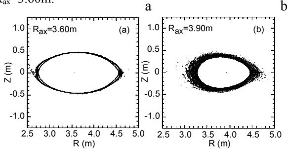
Fig.1. Ergodic layer structures at horizontal cross-section of  $R_{ax}=3.60\text{m}$  (a) and  $3.90\text{m}$  (b)
