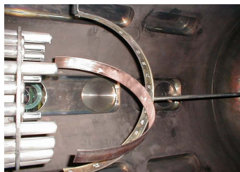
Fig. 1. Internal view of the PF-1000 experimental chamber, which shows a semicircle support with a rotating shield
