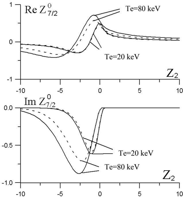
Fig. 2 Weakly relativistic (solid-line) and exact (dash-line) PDFs for  $q = 7/2$  and  $N_{||} = 0.3$  for temperatures  $T_e = 20\text{keV}$  and  $T_e = 80\text{keV}$
