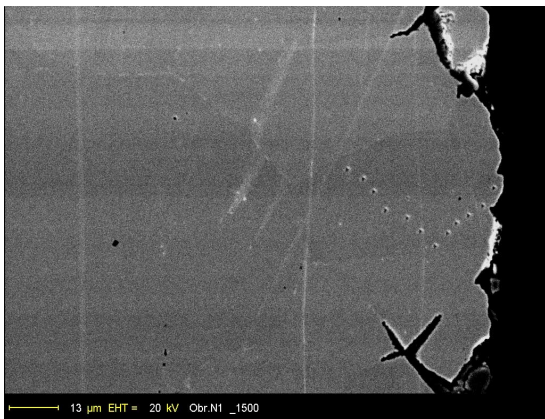
Fig. 16. Surface layer of the alloy A irradiated in salt with E_d=64\text{ eV/at} . Intercrystalline cracks and indenter imprints are seen
