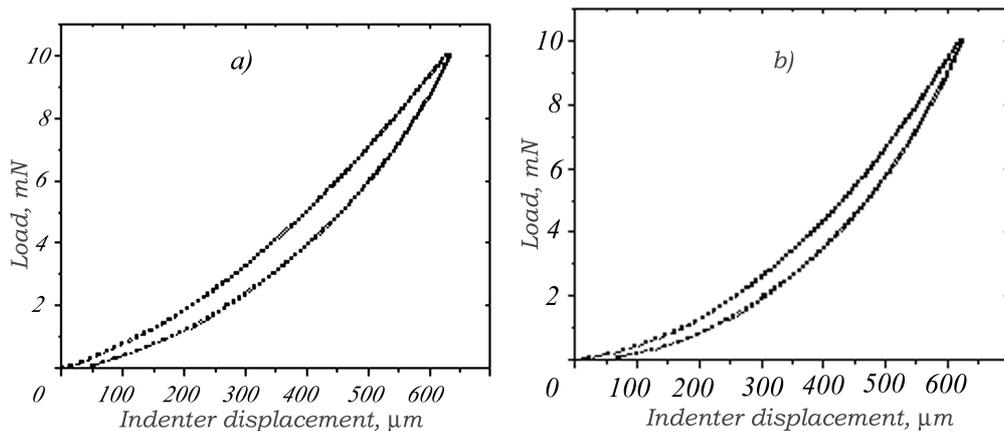
Fig. 2. Loading and unloading curves for carbon-carbon composite materials after electron beam irradiation in a sodium fluoride – zirconium fluoride melt for 700 h at 650 °C: (a) beam entrance (5066 MeV/atom), (b) beam exit (64 MeV/atom)
