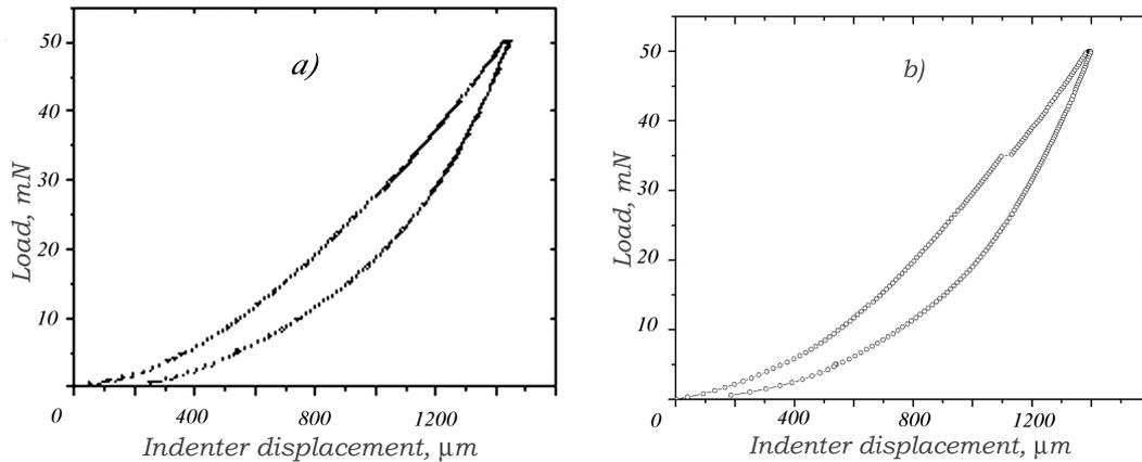
Fig. 1. Loading and unloading curves for carbon-carbon composite materials without contact with fluoride melt and without irradiation: a – sample not tightened with pyrocarbon; b – sample tightened with pyrocarbon
