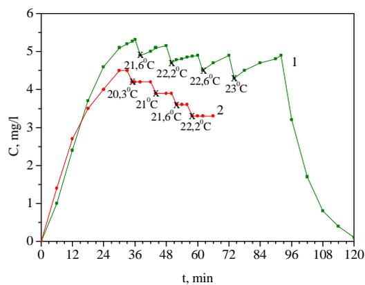
Fig.6. Solubility of ozone in the water with the periodic start of ultrasonic generator. Sterilizations of leaves
