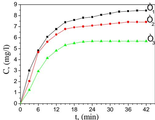
Fig. 3. Solubility of ozone in the distilled water depending on the time; water temperature: 1 - 13° C, 2 - 17.5° C, 3- 24° C; concentration of ozone-air mixture is constant (30 mg/l)
