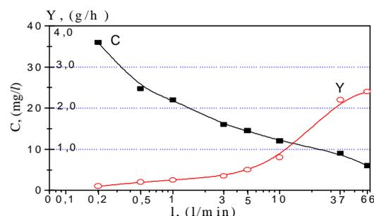
Fig.2. Characteristics of ozone generator with glass enamel dielectric: C – ozone concentration, Y – yield rate, l – air flow rate
