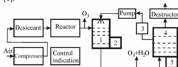
Fig.1. The block diagram of the sterilizer: 1 - mixer, 2 - thermoelectric module, 3 - UV indicator ozone, 4 - sterilization camera, 5 - ultrasonic generator
