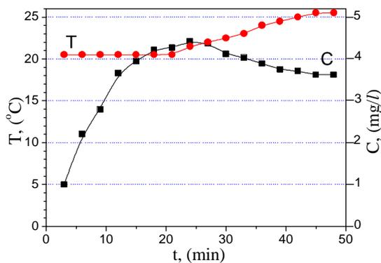
Fig. 4. Dynamics of a change of ozone concentration in the dependence on the water temperature,  $P = 0,07 \text{ atm}$ ,  $U = 300 \text{ V}$ ,  $\lambda = 0,3 \text{ l/min}$
