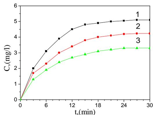
Fig. 5. Solubility of ozone in the distilled water depending on time, with different concentration of ozone at the output of the reactor: 1 – 30 mg/l, 2 – 25 mg/l, 3 – 20 mg/l
