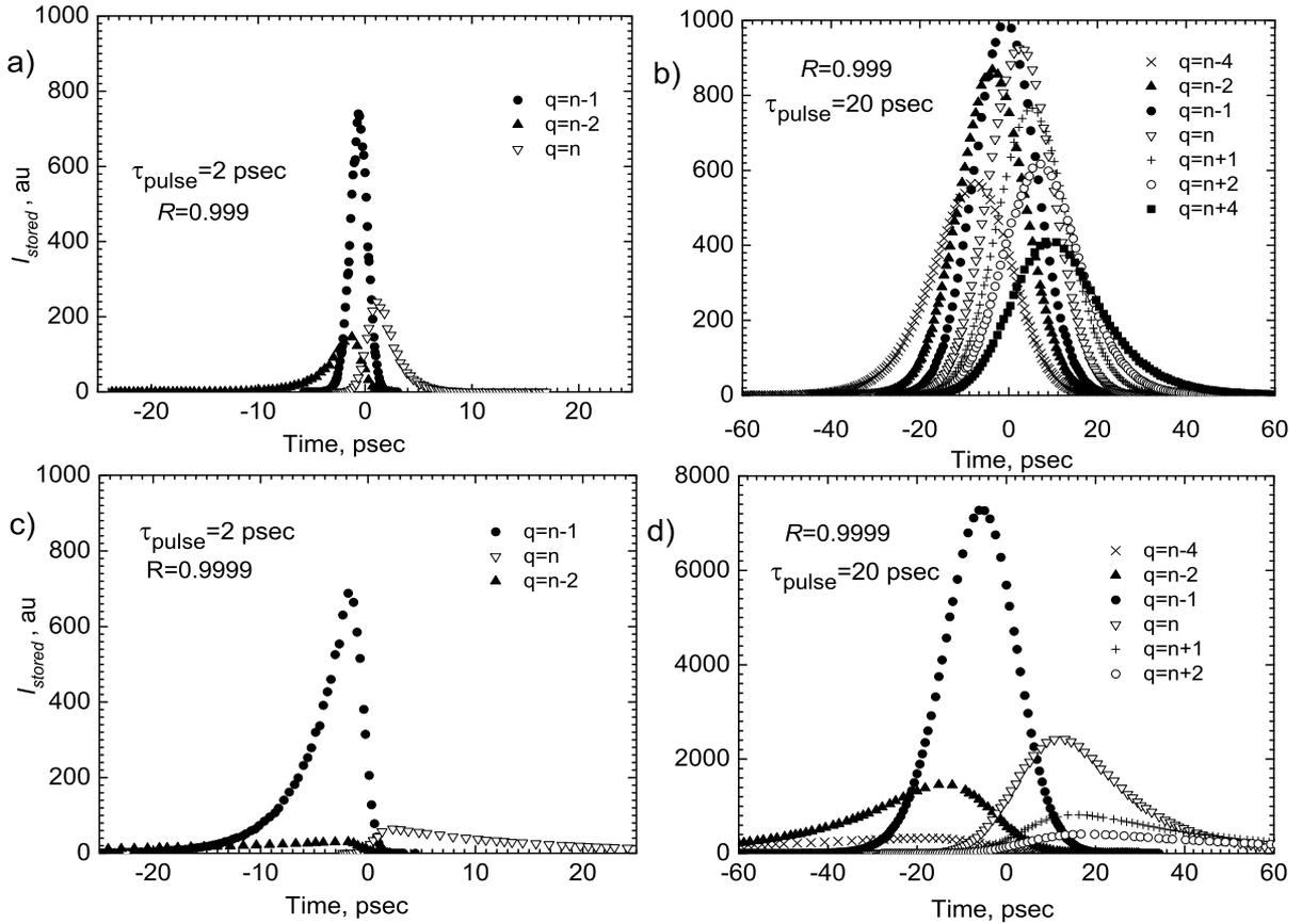
**Fig. 5.** Time profiles of the 2 ps (a, c) and 20 ps (b, d) laser pulse stored in the PSC with medium-reflectivity (a, b) and high-reflectivity (c, d) mirrors. The family of curves in each picture corresponds to different shifts between longitudinal indices of the laser mode and locked PSC mode
