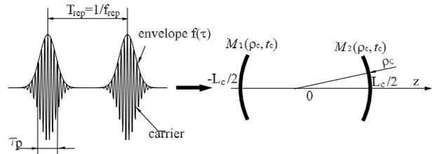
**Fig. 2.** The laser pulse structure and the PSC parameters
