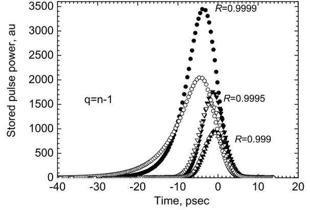
**Fig. 4.** Time profiles of the 7 ps laser pulse stored in 0.42 m PSC. Solid symbols correspond to  $\rho_l=41.7$  m, open symbols refer to  $\rho_l=3.2$  m
