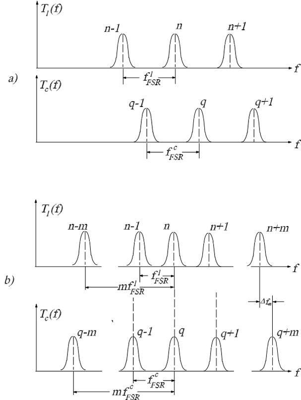
**Fig. 1.** Schematic spectra (frequency combs) of the laser cavity modes and PSC modes: a)  $L_l = L_c$ , no mode locking; b) after adjusting PSC length ( $L_l \neq L_c$ ) for mode locking ( $f_n^l = f_q^c$ )
