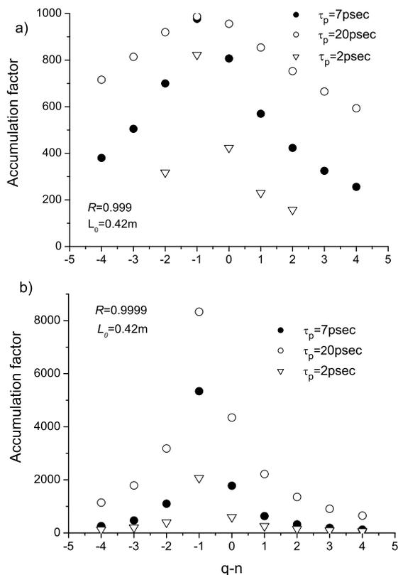
**Fig. 6.** Power gain factor as a function of the cavity mode shift  $q-n$  for medium-reflectivity mirrors (a) and high-reflectivity mirrors (b)
