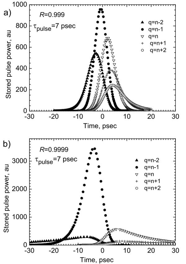
**Fig. 3.** Time profiles of the 7 ps laser pulse stored in 0.42 m PSC with different mirror reflectivity: a)  $R = 0.999$ ; b)  $R = 0.9999$
