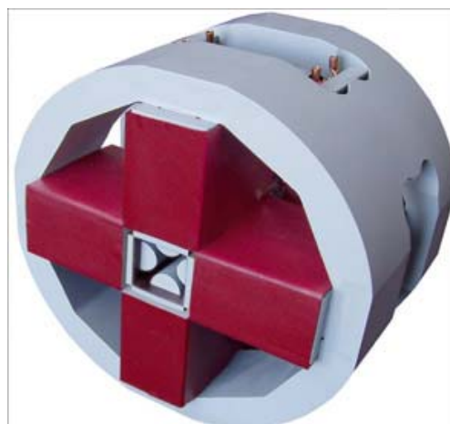
Fig. 7. Doublet of magnetic quadrupole lenses of new design
