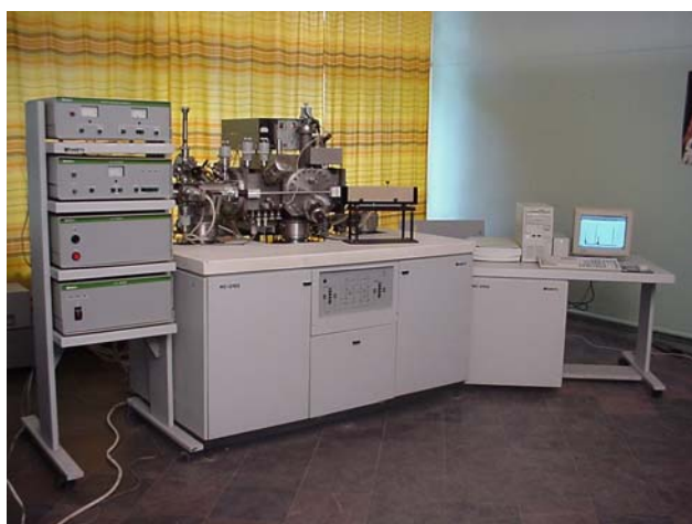
Fig. 9. Laser isotope mass-spectrometer with coordinate-sensitive detector
