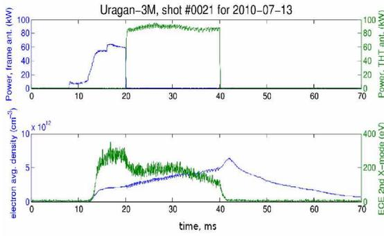
Fig. 2. Temporal evolution of the injected power of the both RF antennae (top) and electron average density radiative temperature (bottom)
