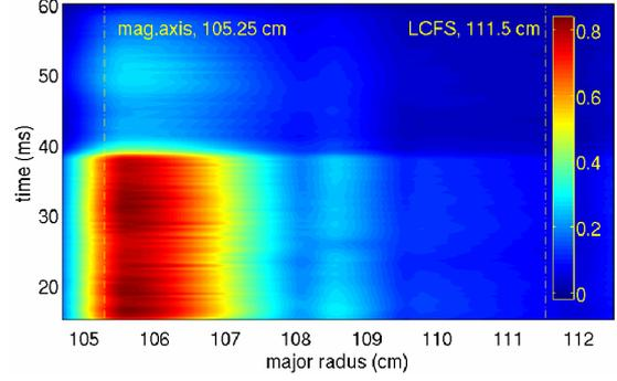
Fig. 3. 2-D Temporal evolution of the electron temperature profile (colored levels of temperature are in the keV)
