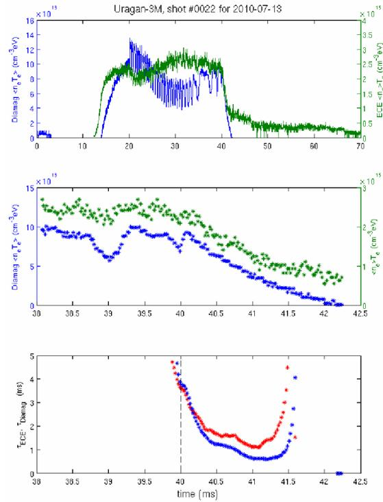
Fig. 4. Temporal evolution of the plasma pressure from local ECE and net diamagnetic measurements (top) their “zoomed” parts for the time of RF heating switch-off (middle) and corresponding energy confinement times
