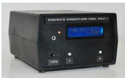
Fig. 2. Meter based on corona discharge
