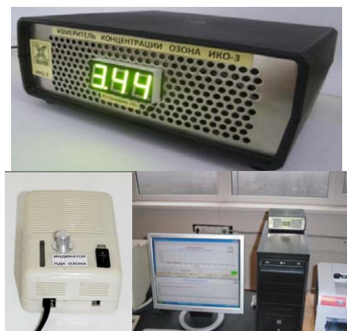
Fig. 3. Semiconductor MAC ozone meter
