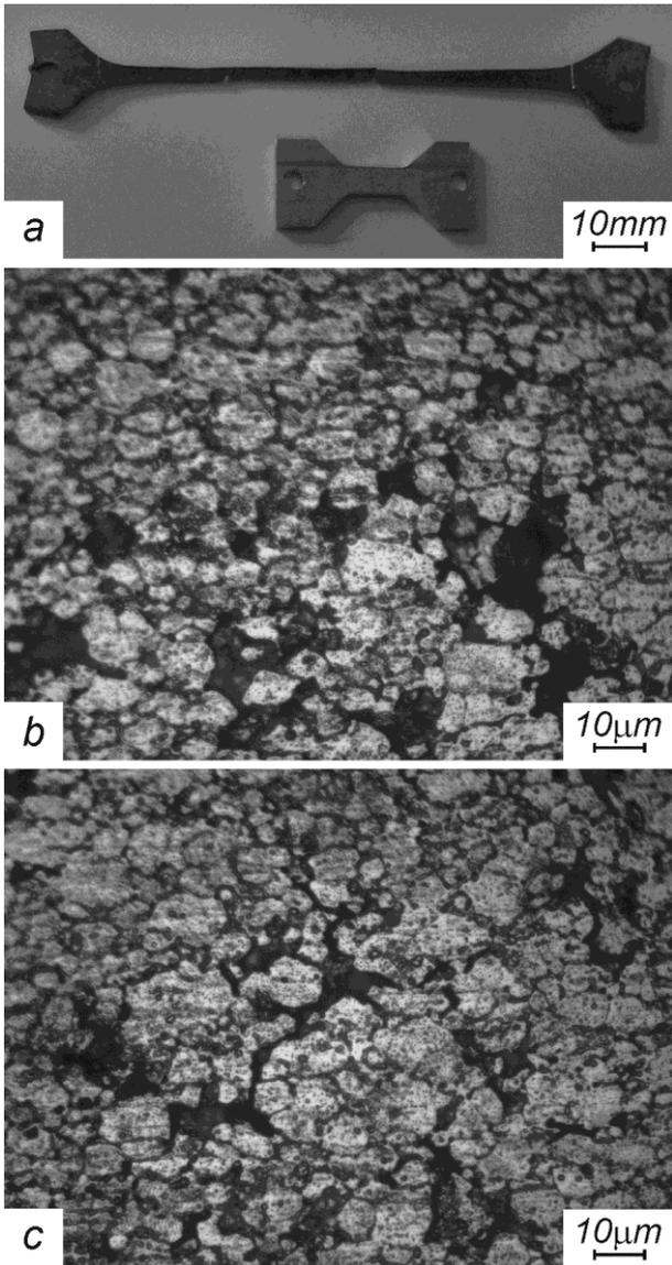
Fig. 3. a – general view of the specimen of alloy 01420T, superplastically deformed to failure in optimal conditions compared to the initial specimen; b and c – views of microstructure of the working part of the specimen deformed to failure in optimal conditions. Horizontal tensile direction. Light microscopy
