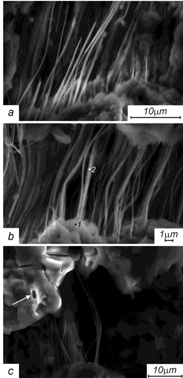
Fig. 4. a and b – types of fibrous structures in the working part of the specimens of alloy 01420T, deformed to failure in optimal conditions of high-temperature superplasticity. Numbers 1 and 2 are the locations in which the chemical composition of the fiber was determined; c – view of the oxidized surface of the grains, tubular cavity and oxidized fibrous structures in the working part of the specimen. The arrow points to the tubular cavity
