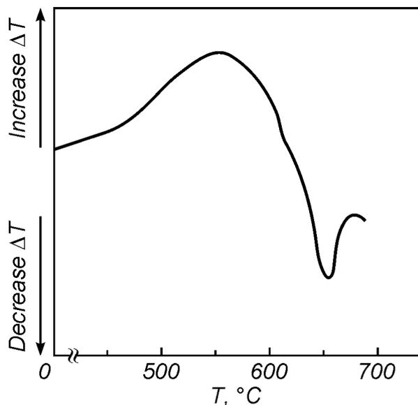
Fig. 5. Extract of differential thermal analysis curve of the specimen of the alloy 01420T in the temperature range 450...680 °C. Optimal temperature of high-temperature structural superplasticity of alloy 01420T  $T = 520$  °C
