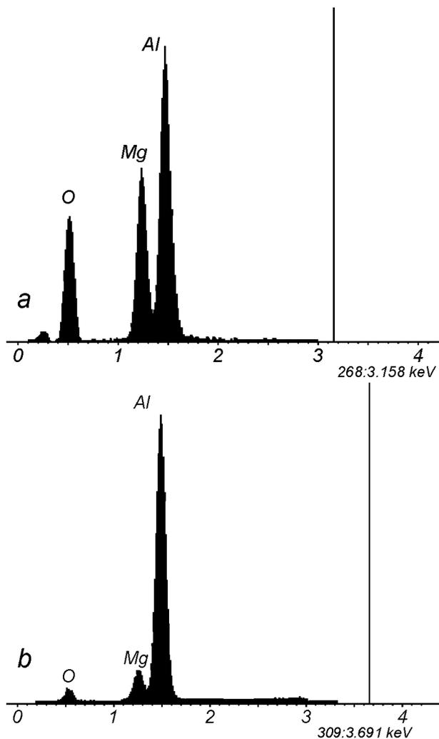
Fig. 6. Energy spectra of the characteristic X-ray that is received from the fiber sections formed during superplastic deformation of the alloy of the specimen 01420T: a - from fiber section, which is located near the place of fixing the fiber to the cavity wall (at the base of the fiber (Fig.4b, point 1), b - the portion of fiber which is located in the middle portion of fiber (Fig. 4,b, point 2)
