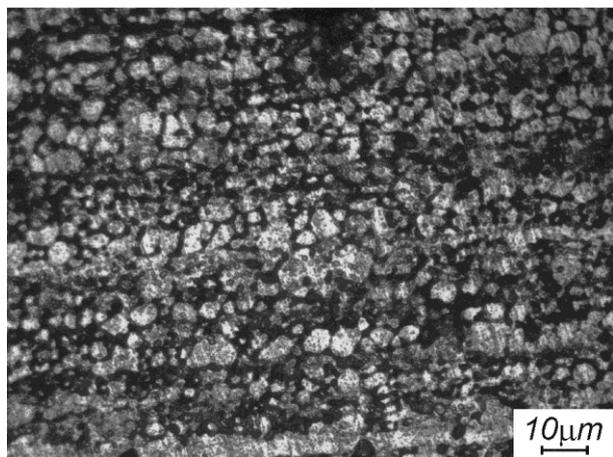
Fig. 1. The initial structure of the specimens of alloy 01420T. Light microscopy
