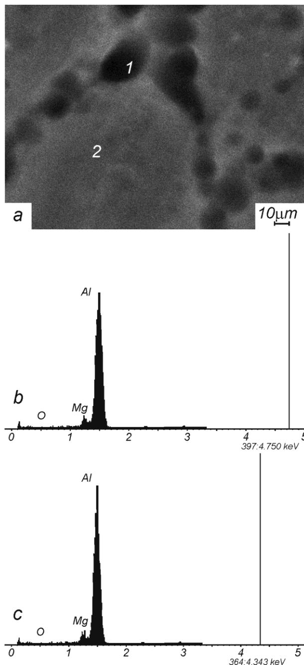
Fig. 2. a – typical view of an area of the working part of the alloy 01420T specimen prepared for mechanical testing (REM); energy spectra of the characteristic X-ray: b – spectrum resulting from point 1 at the grain boundary; c – spectrum resulting from point 2 in the middle of grain
