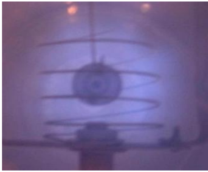
Fig. 2. Finishing ion cleaning with HF-generator in Ar at P_{Ar} = (1...5) \cdot 10^{-1} Pa, U_{cm HF} = (-0.7...1) kV
