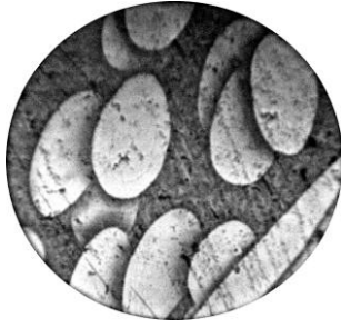
Fig. 7. Treated areas with uniform intensity distribution of the laser radiation
