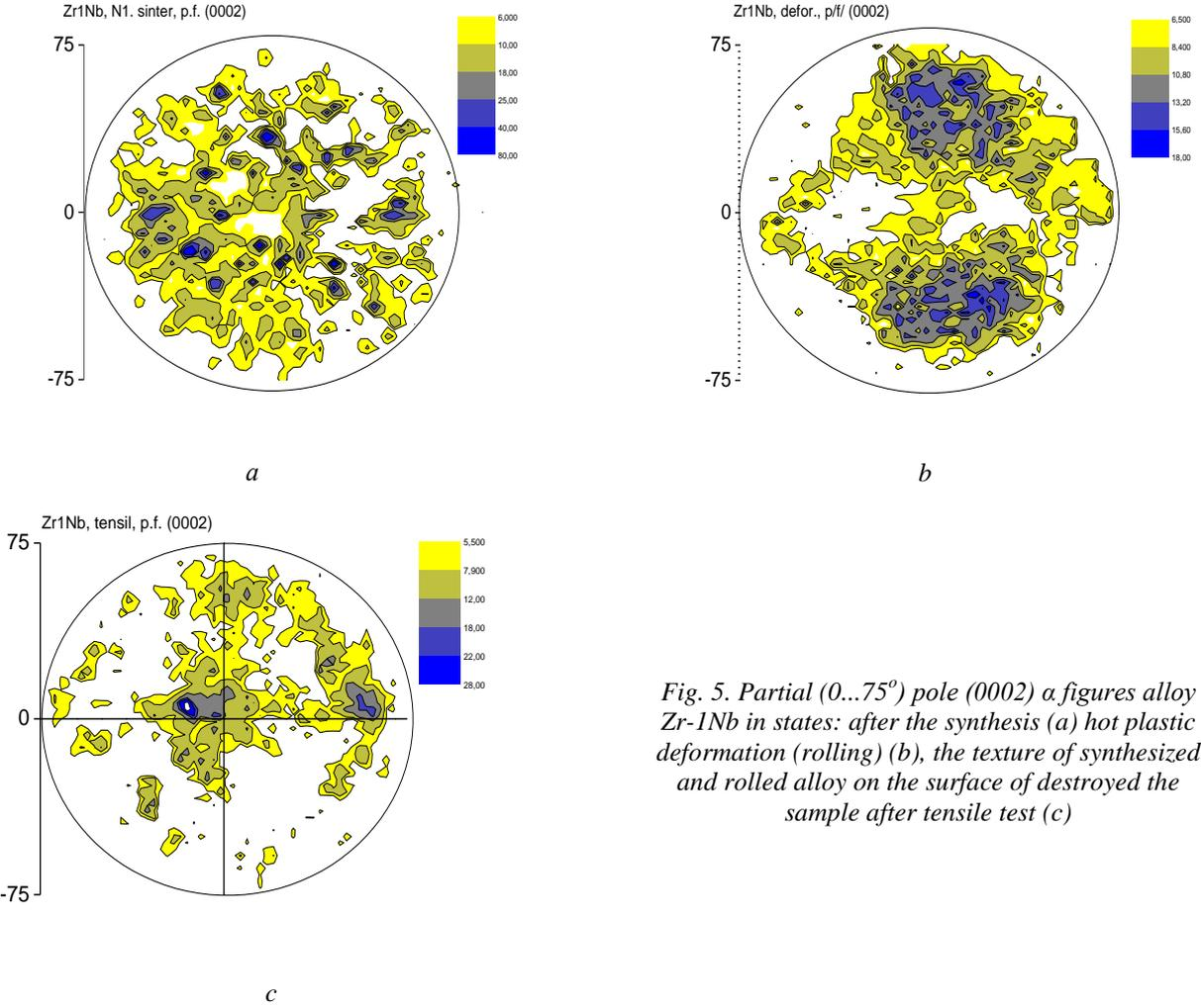
Fig. 5. Partial (0...75°) pole (0002) a figures alloy Zr-1Nb in states: after the synthesis (a) hot plastic deformation (rolling) (b), the texture of synthesized and rolled alloy on the surface of destroyed the sample after tensile test (c)
