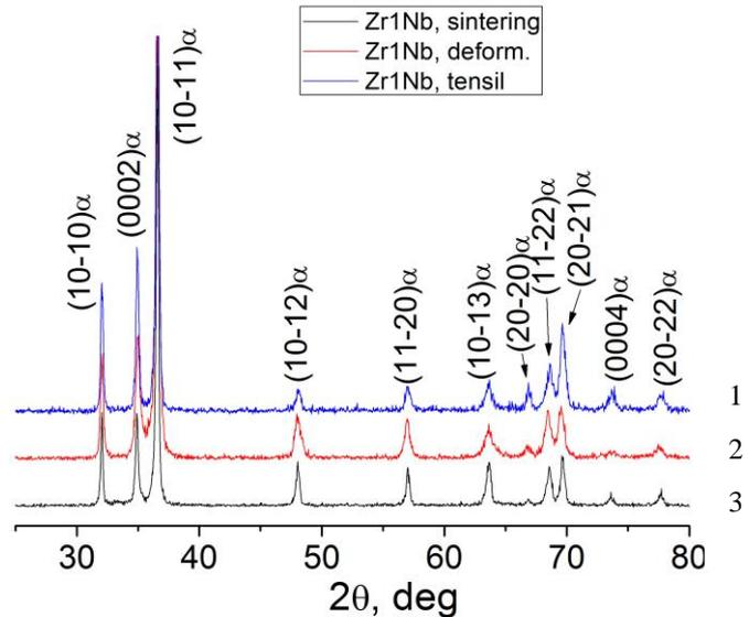
Fig. 4. Radiographs of the Zr-1Nb alloy in states after: sintering (1), deformation (2) and after tensile test (3)
