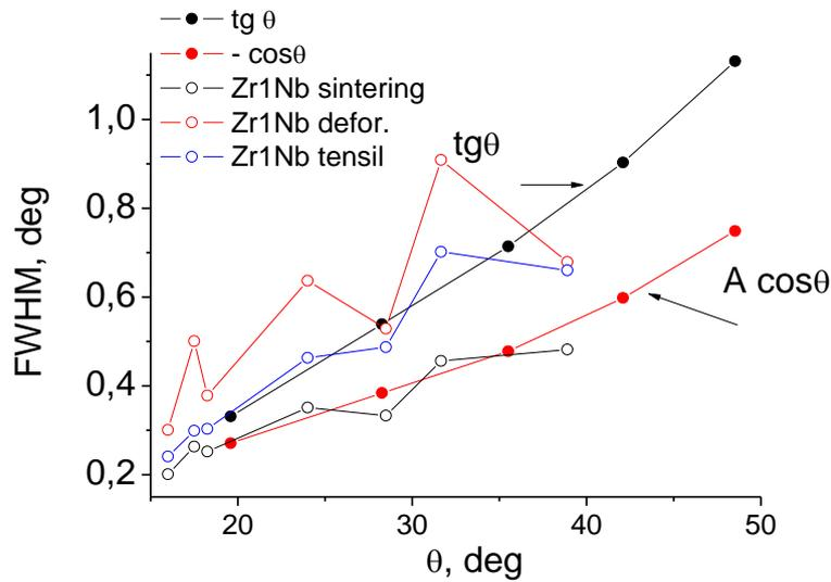
Fig. 6. The dependence of the broadening of the diffraction lines of  $\alpha$ -phase (FWHM) on the angle of reflection  $\theta$
