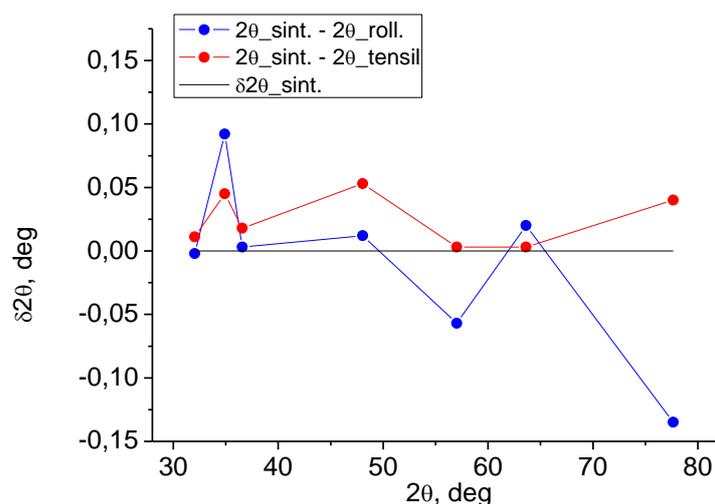
Fig. 8. The displacement of diffraction reflections of angles  $\delta 2\theta$  alloy Zr-1Nb: after rolling (blue line) and after tensile (red line)
