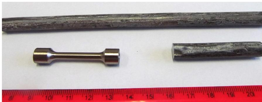
*Fig. 2. Rods Zr-1% Nb alloy, obtained by rolling, and the sample was machined from a rod for mechanical tests*
