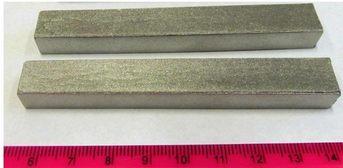
*Fig. 1. Samples of the sintered Zr-1%Nb alloy*
