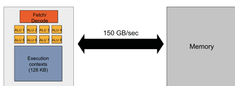
Fig.5. Structure of direct memory addressing in the GPU architecture
