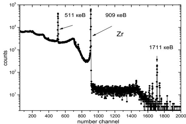
**Fig.3.** The  $\gamma$ -spectrum of  $\text{ZrO}_2$  nanoparticles
