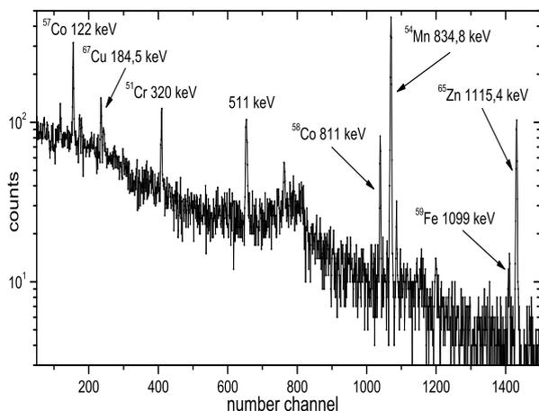
**Fig.1.** The  $\gamma$ -spectrum of nanoparticles  $\text{Fe}_2\text{O}_3$
