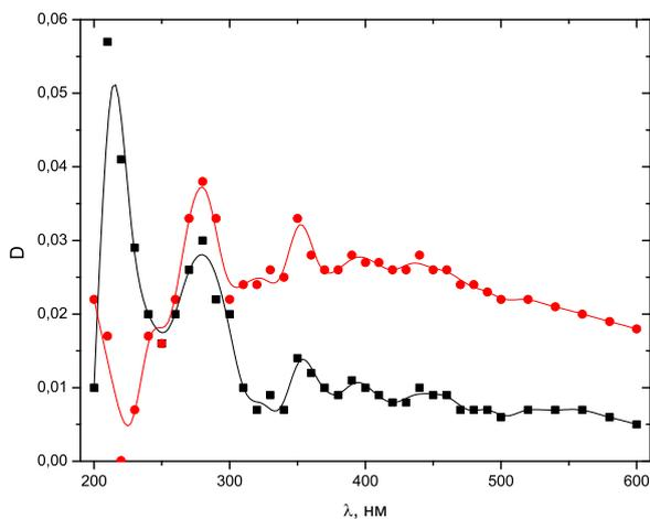
**Fig.5.** The absorption spectrum of the methane conversion with using as catalysts  $\gamma$ -activated ZrO<sub>2</sub> nanoparticles
