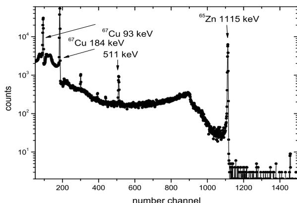
**Fig.2.** The  $\gamma$ -spectrum of ZnO nanoparticles
