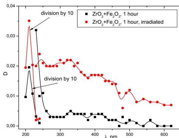
**Fig.6.** The absorption spectrum of methane conversion products with using as catalysts  $\gamma$ -activated nanoparticles of ZrO<sub>2</sub>/Fe<sub>2</sub>O<sub>3</sub>
