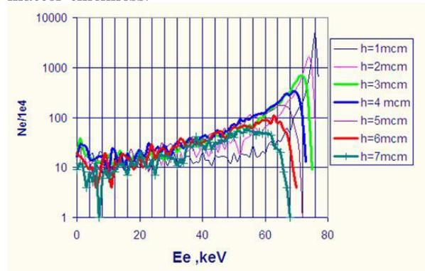
**Fig.4.** Electron spectrum output dependence on gadolinium thickness. Primary electron energy  $E_e = 78$  keV
