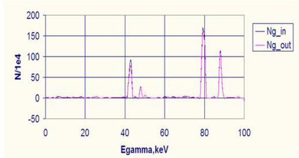
**Fig.5.**  $\gamma$ -quantum absorption in Si-detector in the energy range up to  $100 keV$
