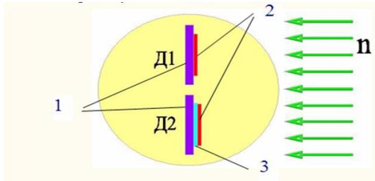
**Fig. 1.** Two detector model scheme. 1 -- PSD; 2 – gadolinium converters; 3 — polyethylene screen
