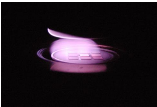
Fig. 4. A photograph of a discharge in a hydrogen medium with addition of 0.75% methane at a pressure of 60 mm Hg and a discharge current of 5.2 A in the case a grounded substrate holder with a diameter of 62 mm; exposures are the following: a – 1/1000 s; b – 1/100 s
