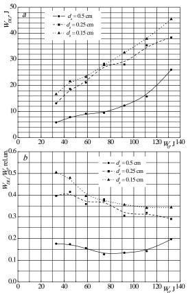
Fig. 4. Dependence of the energy (a) and the specific energy (b), released in the discharge in the 1<sup>st</sup> halfperiod, on the initial stored energy for different high-voltage electrode diameters
