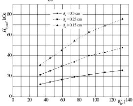
Fig. 6. Dependence of the magnetic field strength of the maximum discharge current on the initial stored energy for different high-voltage electrode diameters
