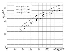
Fig. 3. Dependence of the maximum discharge current on the initial stored energy for different high-voltage electrode diameters
