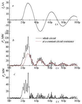
Fig. 2. Dynamics of the discharge current (a), the active power generated in the circuit (b) and inputted into the discharge (c) at a charging voltage  $V_0 = 12 \text{ kV}$ and the high-voltage electrode diameter  $d_a = 0.25 \text{ cm}$
