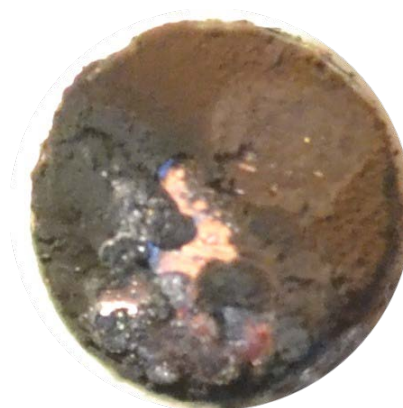
Fig. 13. Ni (anode in bottom position) and Cu (cathode in upper position)
