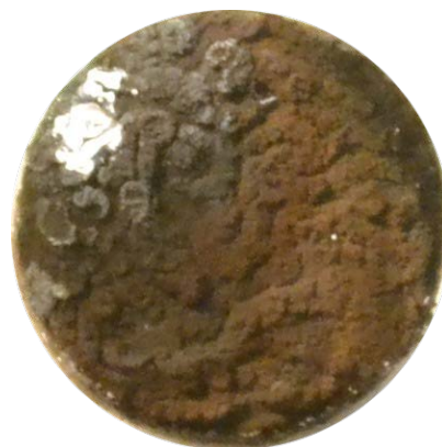
Fig. 12. Ni (anode in upper position) and Cu (cathode in bottom position)
