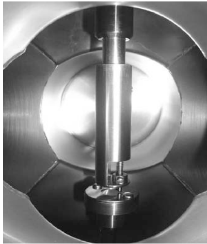
Fig. 1. The cathode-holder with the sample and anode in the vacuum chamber
