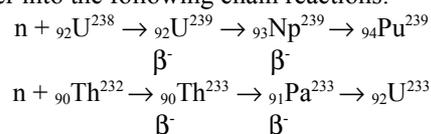
These two reactions have opened up a real possibility for nuclear fuel breeding in the progress of chain reaction.
