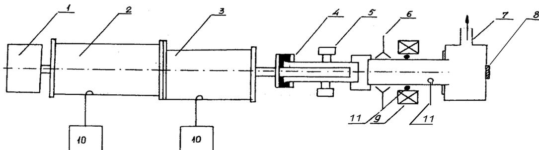
Fig.3. Scheme of the installation. (1) proton injector; (2) initial stage of accelerator; (3) final stage; (4) plasma gun; (5) gas valve; (6) horn antenna; (7) chamber; (8) luminescence screen; (9) solenoid; (10) RF sources; (11) magnetic field probes.
