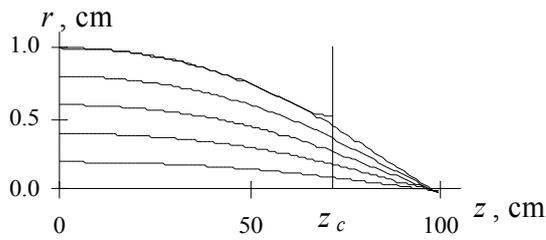
Fig. 2. The trajectories of the focused protons in the optimized magnetic field.
