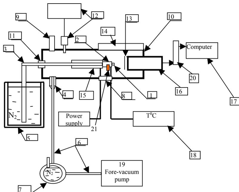
Fig.1. The scheme of the pyroelectric X-ray generator
