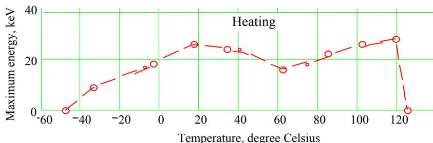
Fig. 6. Maximum energy of X-rays versus crystal temperature at heating conditions
