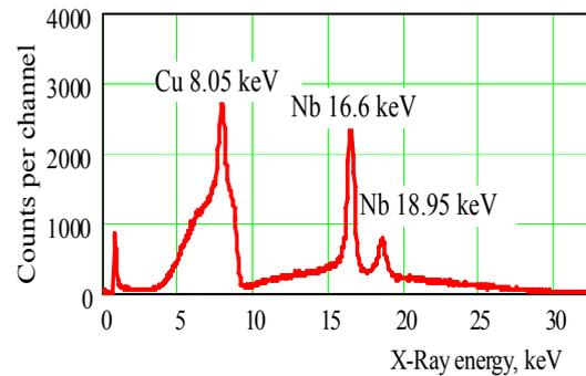
Fig.4. X-ray radiation spectrum measured with Cu foil and crystal elements during  $\text{LiNbO}_3$  crystal heating. The distance between the crystal and the copper foil is  $7.5 \text{ mm}$ . The total number of counts in the spectrum is  $4.975 \cdot 10^5$  for 8 minutes. The residual air pressure in the vacuum chamber, which accommodates the crystal, is measured to be  $25 \text{ mTorr}$
