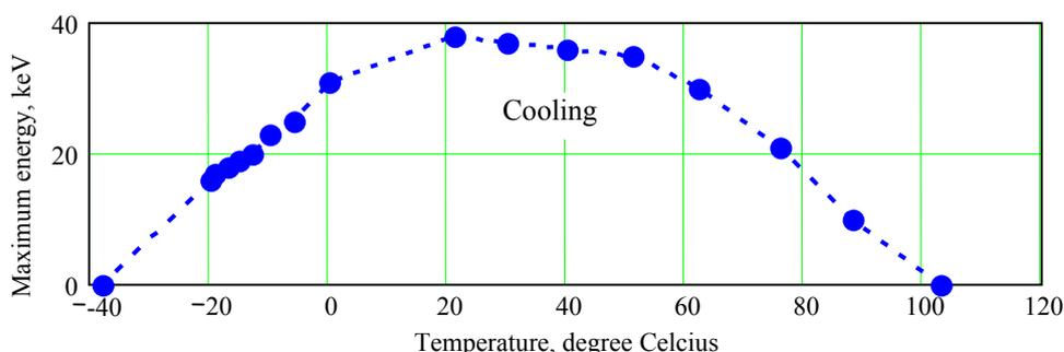
Fig.7. Maximum energy of X-rays versus crystal temperature at cooling conditions
