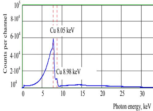
Fig.2. X-ray radiation spectrum measured with Cu target thickness  $20 \mu\text{m}$  at  $\text{LiNbO}_3$  crystal cooling. The value of one channel is  $0.036 \text{ keV}$ . The distance between the crystal and the copper foil is  $7.5 \text{ mm}$ . The total number of counts in the spectrum is  $8.391 \cdot 10^6$  for 16 minutes. The residual air pressure in the vacuum chamber is measured to be  $25 \text{ mTorr}$
