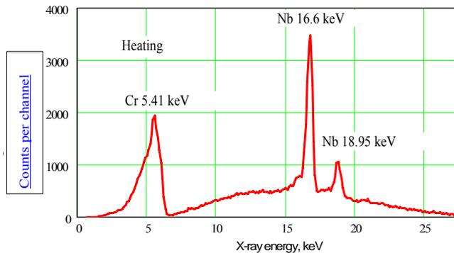
Fig.5. X-ray radiation spectrum measured with Cr target thickness  $18 \mu\text{m}$  at  $\text{LiNbO}_3$  crystal heating for one minute
