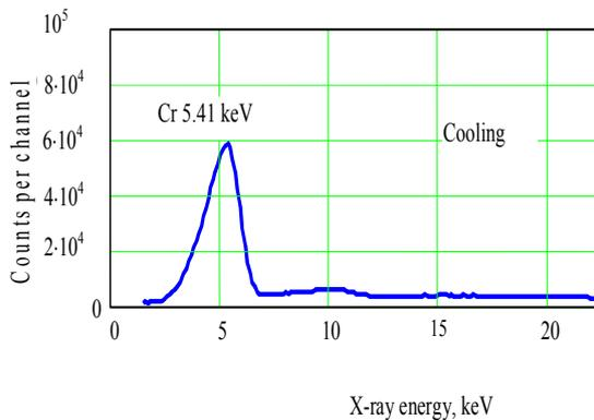
Fig. 3. X-ray radiation spectrum measured with Cr target thickness  $18 \mu\text{m}$  at  $\text{LiNbO}_3$  crystal cooling for one minute
