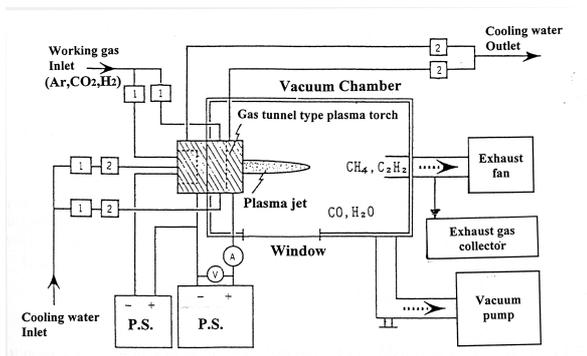
Fig.6. High energy plasma system for the recombination of carbon dioxide
