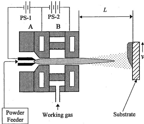
Fig.1. Schematic of the gas tunnel type plasma spraying torch
