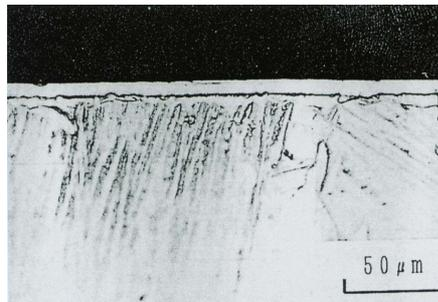
Fig.5. Microphotograph of cross section of TiN film. Ti substrate irradiated at  $L=70\text{mm}$  when  $P=20 \text{ kW}$
