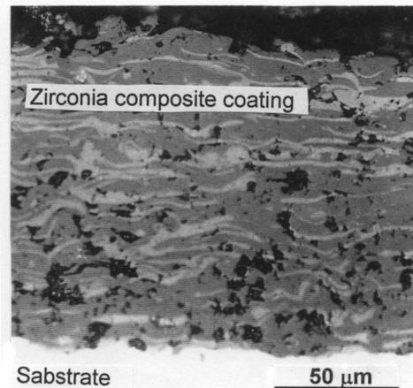
Fig. 3. Microphotograph of cross section of zirconia composite coating. The traverse number was 30 time traverse. Sprayed at L=40mm when P=25 kW
