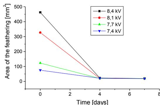
Fig.3. Atmospheric corona discharge PES fabric modification effect aging expressed in the feathering spot size time changes for different input power values
