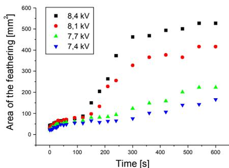
Fig. 1. Time dependence of the fabric moistened and feathering area
