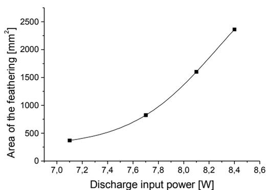
Fig. 2. Discharge input power dependence of moistened and feathering area
