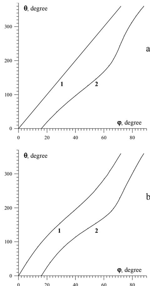
Fig.1 The winding laws of the main 1a)-  $\theta(\varphi)=5\varphi$ , 1b)-  $\theta(\varphi)=2\text{arctg}(1.291\text{tg}(2.5\varphi))$  and auxiliary 2a), 2b) helical coils along the length of the helical pitch
