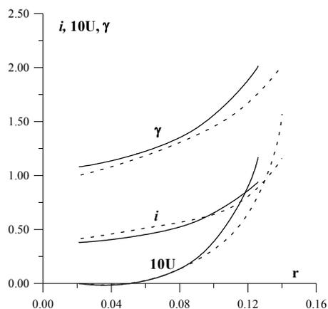
Fig.3. The field ripple  $\gamma$ , rotational transform angle  $i$  (in  $2\pi$  units), magnetic hill value  $U$  versus the average magnetic surface radius  $r$  for shifted (solid lines) and unshifted (dotted lines) magnetic surfaces
