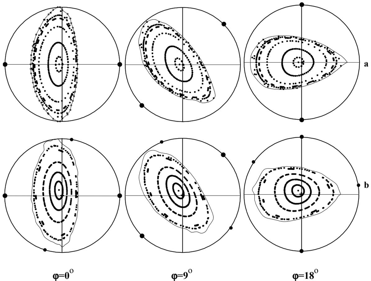
Fig.2 Cross-sections of magnetic surfaces (dotted lines) and equiconnects (thin solid lines) within the half period of magnetic field: a) the SPC is currentless, b) the SPC is turned on. Large solid points are the main helical base line cross-sections, smaller solid points are the auxiliary helical base line cross-sections
