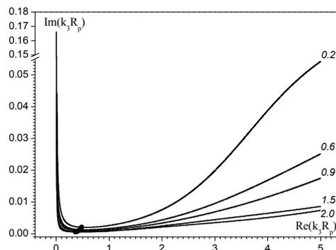
Fig. 4. The dependence of the SW attenuation coefficient  $\alpha$  on the external magnetic field value for radially uniform plasma. The parameters are the same as in Fig. 3
