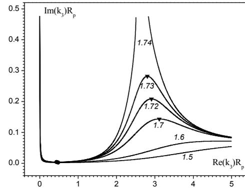
Fig. 2. The dependence of the SW attenuation coefficient  $\alpha$  on the value of the vacuum gap thickness for radially uniform plasma. The parameters are the same as in Fig. 1
