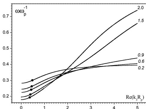
Fig. 3. The dependence of the SW phase properties on the external magnetic field value for radially uniform plasma. Numbers at the curves corresponds to the parameter  $\Omega$  value. Other parameters are equal to  $\delta=0.3$ ,  $\eta=1.5$ ,  $\tilde{\nu}=0.001$ ,  $\varepsilon_d=4.5$ ,  $\sigma=0.3$  and  $m=-1$
