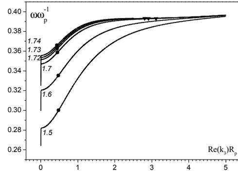
Fig. 1. The dependence of the SW phase properties on the value of the vacuum gap thickness for radially uniform plasma. Numbers at the curves correspond to the parameter  $\eta$  value. Other dimensionless parameters are equal to  $\tilde{\nu} = 0.001$ ,  $\varepsilon_d = 4.5$ ,  $\Omega = 0.2$ ,  $\sigma = 0.3$ ,  $\delta = 0.3$  and  $m = -1$
