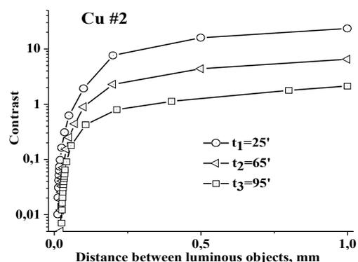
Fig. 7. The image contrast of two objects upon the distance between their opposite points after successive exposures for mirror Cu #2
