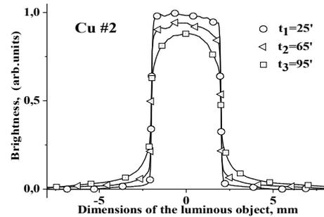
Fig. 5. The set of curves for dependences of light intensity transmitted by the large-grain Cu mirror on the linear size of the light object at successive exposures to ion bombardment
