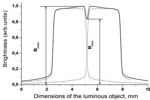
Fig. 3. The scheme of determination of the contrast and the limiting linear (and angle) resolution
