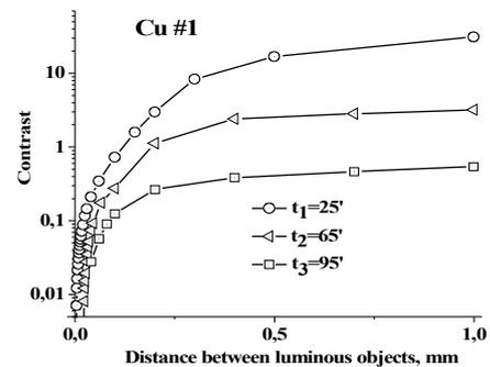
Fig. 6. The image contrast of two objects upon the distance between their opposite points after successive exposures for mirror Cu #1
