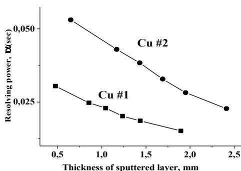
Fig. 8. Degradation of the resolving power of mirror samples Cu #1 and Cu #2 for  $K=0.25$  with increasing the depth of layer eroded by ion sputtering
