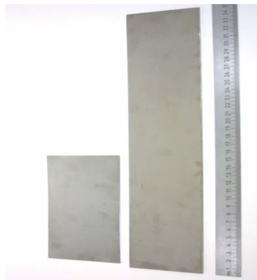
Fig. 7. Plates made of a hafnium ingot smelted from double burden
