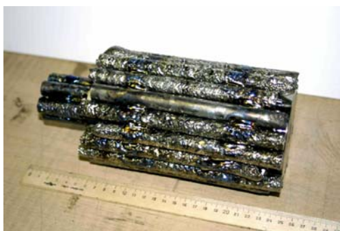
Fig. 4. Double burden (CTH + IH) electrode for VAR
