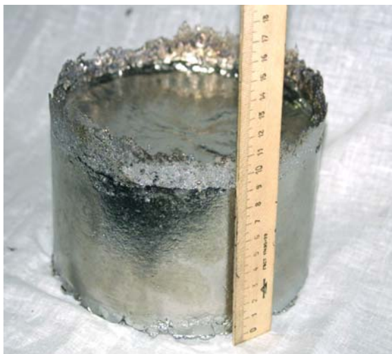
Fig. 6. Pilot ingot 160 mm in diameter weighing 22 kg smelted from double burden (CTH+IH)
