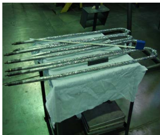
Fig. 1. Iodide hafnium bars produced from melting and deformation processes wastes
