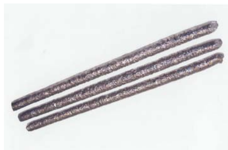
Fig. 3. Hafnium iodide bars HFI-1 grade received in H-3 device
