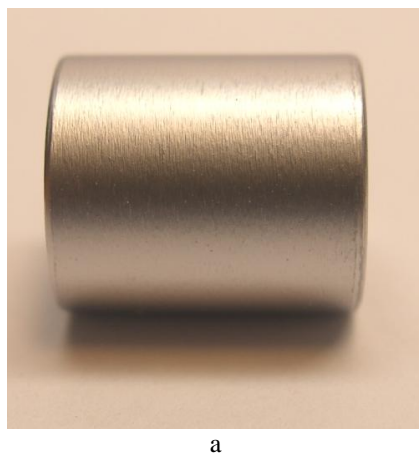
Fig. 1. Photograph of the E110 tube with chromium coating (a) and SEM image of tube metallographic section (b)
