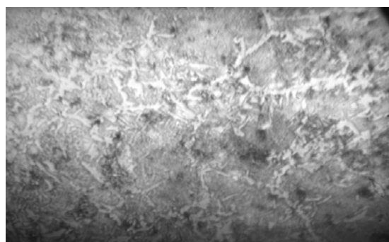
Fig. 5. Boundary layer between hardened and raw areas
