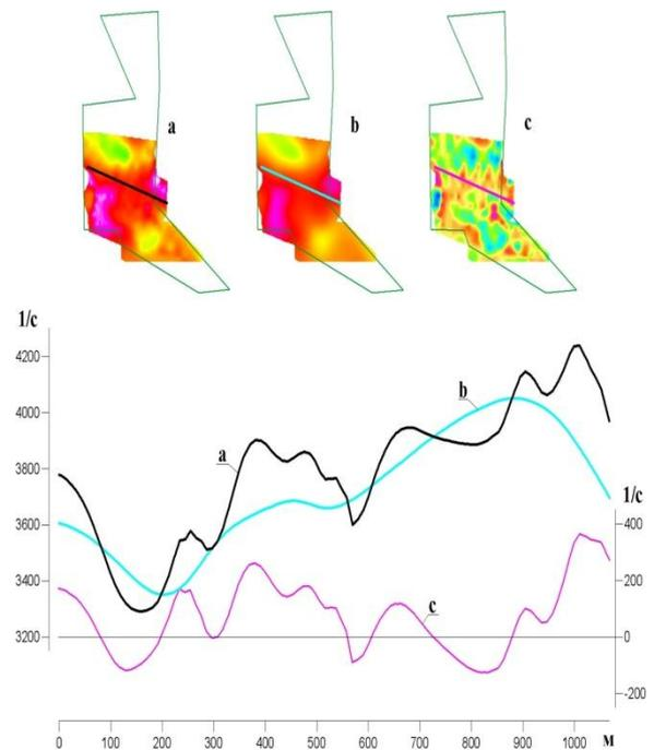
Fig. 4. Graphic of initial (a), average (b) and local component (c) of gamma radiation fields, on area “Red forest”. In the top - position of the line graphs at corresponding maps
