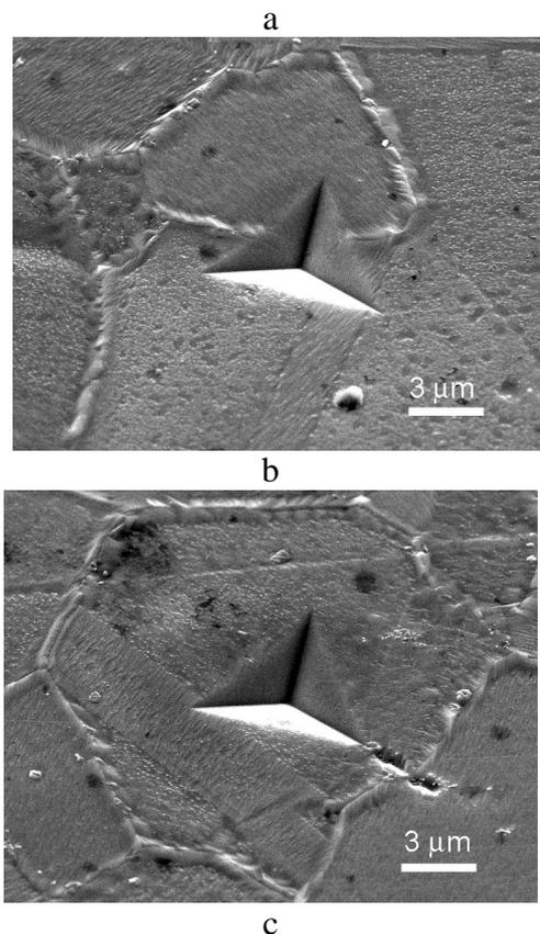
Fig. 4. Hardness of SS316 steel irradiated at 900 K with 1.4 MeV  $\text{Ar}^+$  ions to a dose of  $1 \cdot 10^{17} \text{ cm}^{-2}$  measured on boundary (1) and in grain body (2) (a). Surface of specimen with imprints of indentation # 1 (b) and # 2 (c)
