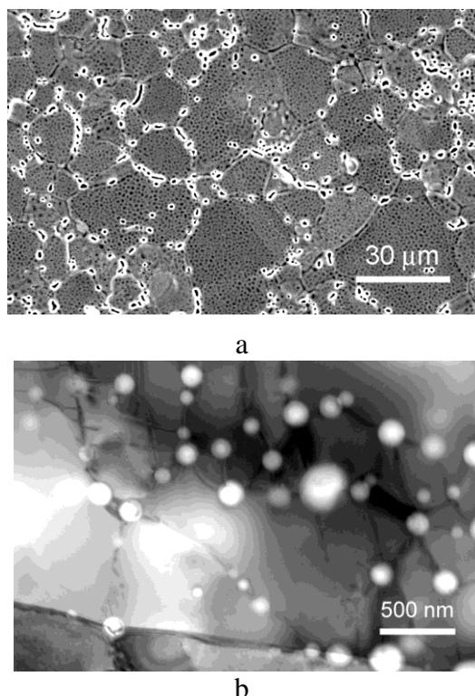
Fig. 5. Microstructure of SS316 steel irradiated at 900 K with 1.4 MeV  $Ar^+$  ions to a dose of  $1 \cdot 10^{17} \text{ cm}^{-2}$  obtained by means of SEM (after electro polishing) (a) and TEM (b)
