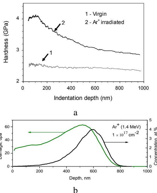
Fig. 6. Profile of hardness of steel 316 for initial (1) and argon irradiated (2) specimens (a); designed profiles of damage and concentrations of argon with energy of irradiation 1.4 MeV to dose  $1 \cdot 10^{17} \text{ cm}^{-2}$  (b)
