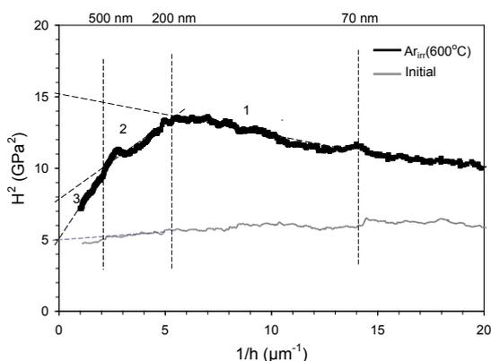
Fig. 7. Dependence of  $H^2 = f(1/h)$  for initial and argon irradiated specimen of steel 316
