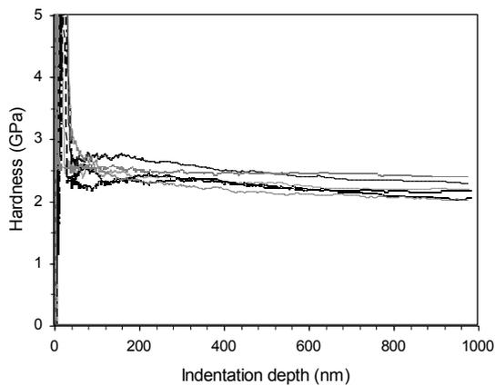
Fig. 3. Dependence of hardness of SS316 steel in initial state from the depth of indenter penetration
