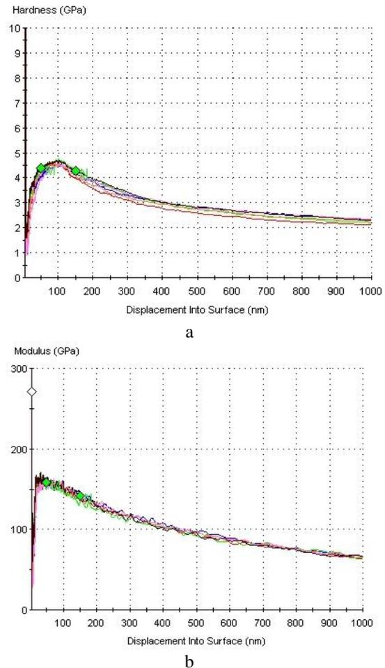
Fig. 2. Hardness (a) and elastic modulus (b) of SS316 steel irradiated with 1.4 MeV Ar<sup>+</sup> ions
