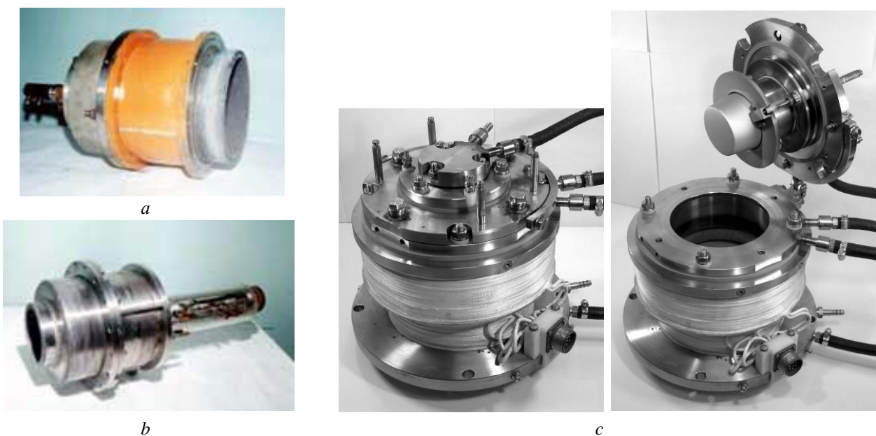
Fig. 11. Faced vacuum arc plasma sources: a – source for equipment of type Bulat-6; b – for deposition of thick coatings; c – source of improved design for facilities of new models
