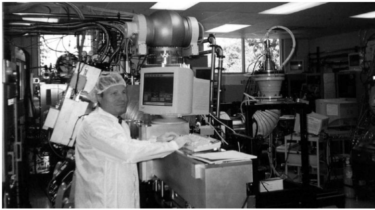
Fig. 9. New-York, USA, 2001 (VEECO Instruments, Inc.). Toroidal filter in complex of industrial equipment for production of elements of recording and reading of information
