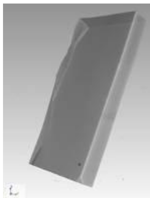
Fig. 5. XRD Tomography of SiC – c
