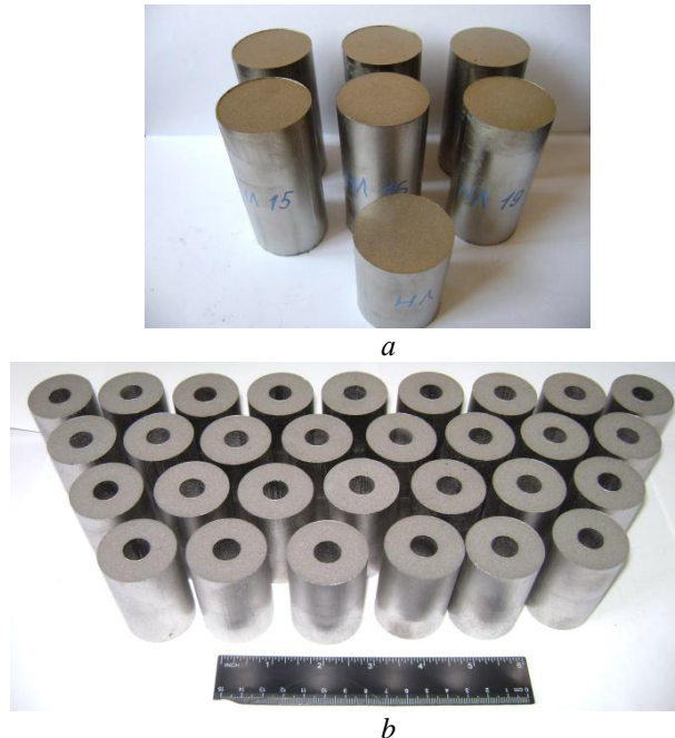
Fig 1. Sintered work pieces for rod a) and pipe b)
