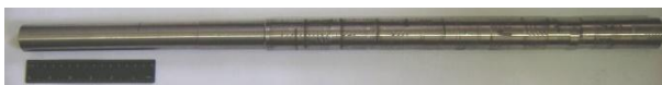
Fig. 5. Rod work piece ( \varnothing 40 mm, length 700 mm) produced using PM and welding methods
