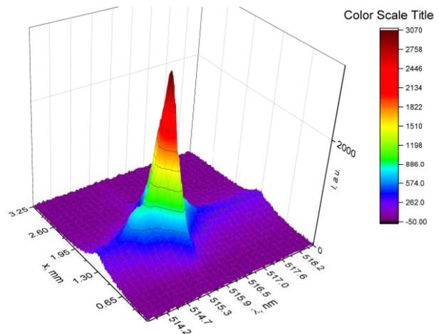
Fig. 4. 3D plot of the Cu I 515.3 nm profile, emitted by the discharge between copper electrodes immersed into deionized water
