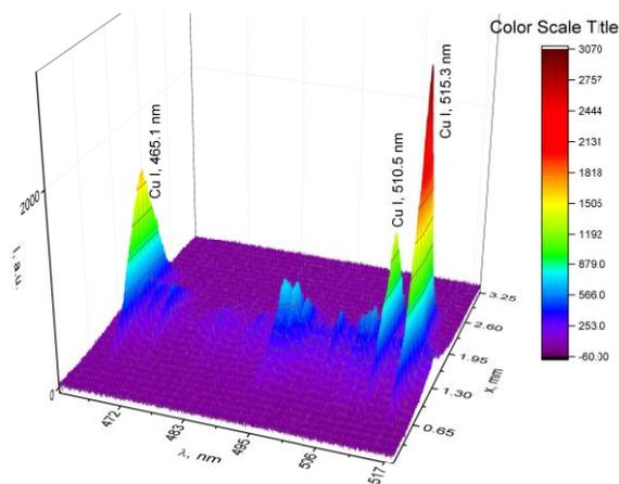
Fig. 3. 3D plot of the emission of the discharge between copper electrodes immersed into deionized water
