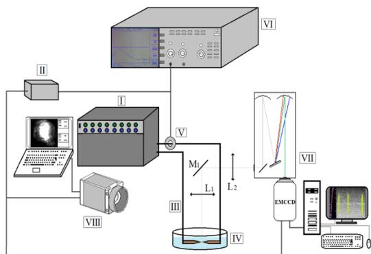
Fig. 1. Experimental setup for the single-pulse underwater electric discharge generation between two electrodes
