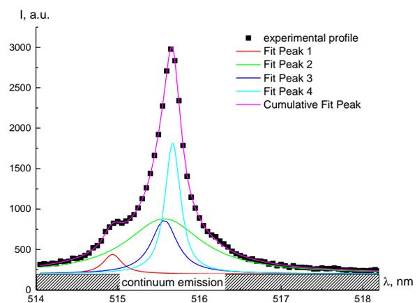
Fig. 5. Observed along discharge axis Cu I 515.3 nm profile, emitted by the discharge between copper electrodes immersed into deionized water
