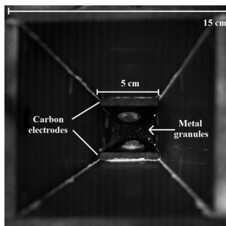
Fig. 2. The top view of the discharge chamber used for the estimation of the spark duration between two metal granules
