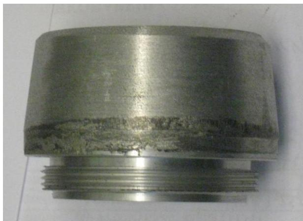
Fig. 1. General view of the cathode before evaporation
