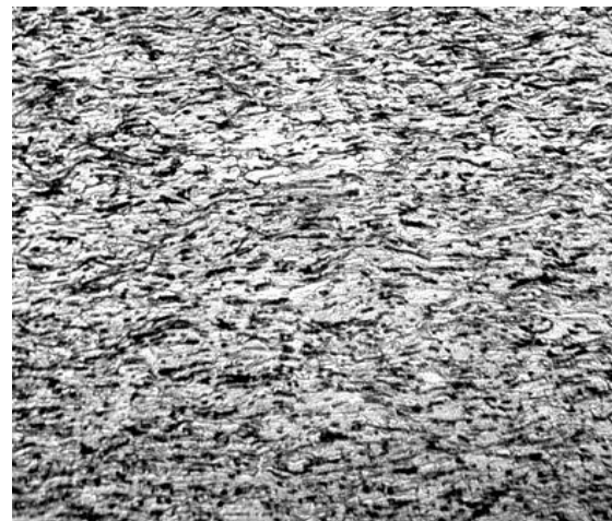
Fig. 6. Microstructure of tubes of finished \varnothing 12.7 \times 0.889 mm size after stress-relief heat treatment ( \times 500 )
