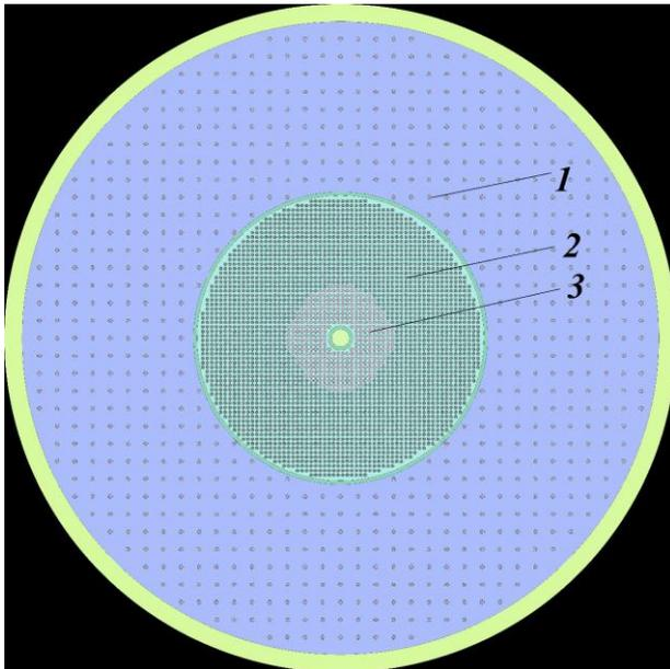
Fig. 8. Heterogeneous (central) layout of fuel elements (Pu+MA) in the core: 1 – thermal zone fuel element with 5% enriched fuel  $\text{UO}_2$ ; 2 – fast zone fuel element with 10% enriched fuel  $\text{UO}_2$ ; 3 – fuel element with fuel Pu+MA
