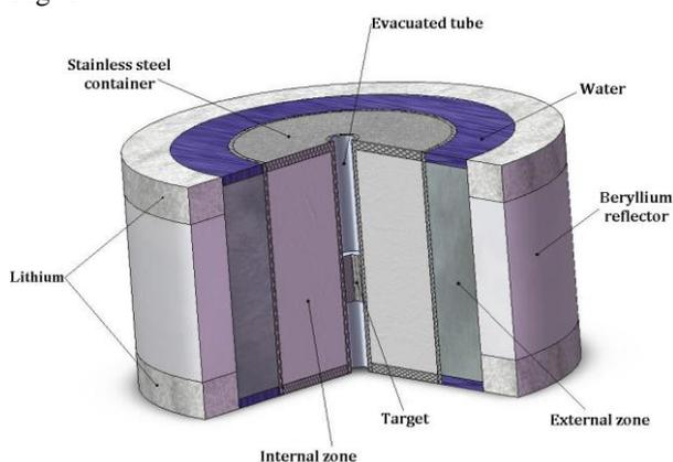
Fig. 1. The general view of a two-zone research subcritical reactor
