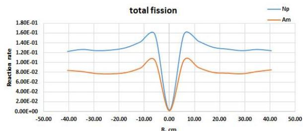
Fig. 5. Distribution of the fission reactions rates for  $^{237}\text{Np}$ ,  $^{243}\text{Am}$  in the inner zone of the subcritical system
