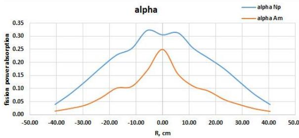
Fig. 7. Distribution of "alpha" for  $^{237}\text{Np}$ ,  $^{243}\text{Am}$  in the inner zone of the subcritical system
