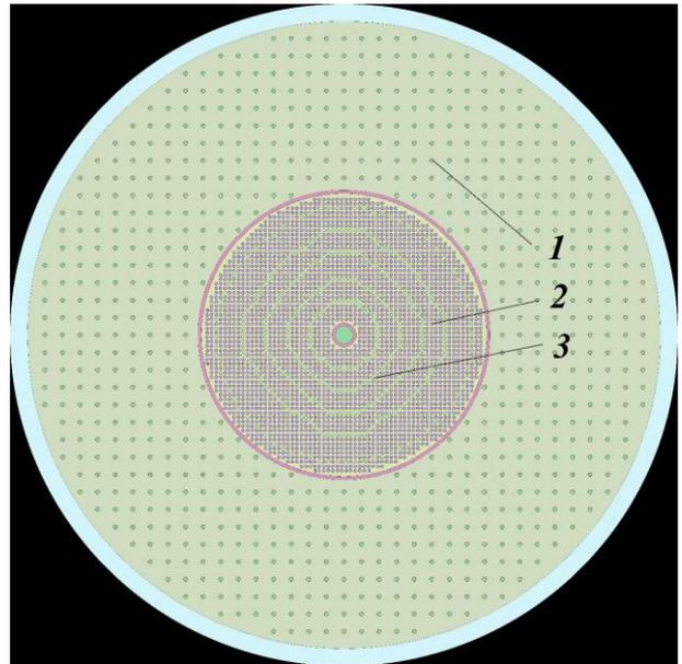
Fig. 9. Homogeneous layout of fuel elements (Pu+MA) in the core: 1 – thermal zone fuel element with 5% enriched fuel  $\text{UO}_2$ ; 2 – fast zone fuel element with 10% enriched fuel  $\text{UO}_2$ ; 3 – fuel element with fuel Pu+MA
