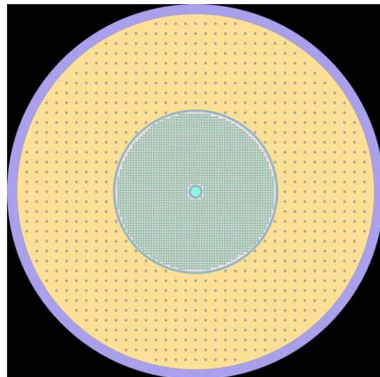
Fig. 3. Cross section of a cylindrical two-zone subcritical system modeled using Serpent code
