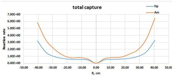
Fig. 6. Distribution of the capture reactions rates for  $^{237}\text{Np}$ ,  $^{243}\text{Am}$  in the inner zone of the subcritical system
