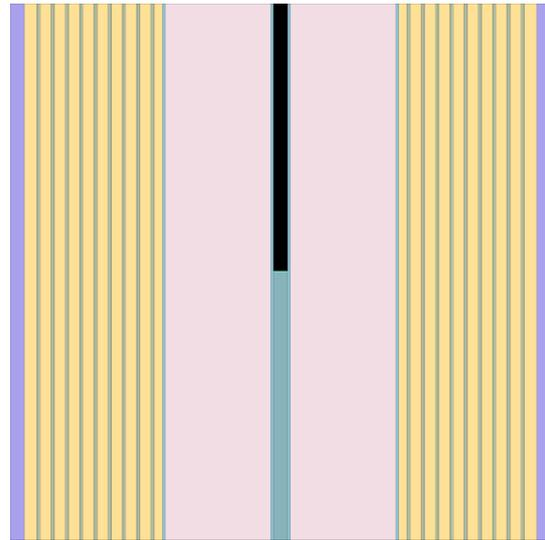
Fig. 2. The vertical cross-section of a cylindrical subcritical system modeled using the Serpent code
