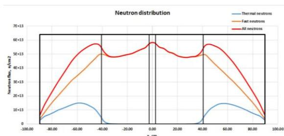
Fig. 4. Distribution of thermal and fast neutrons in the subcritical system
