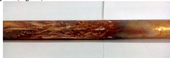
Fig. 12. Cathode spots traces left on the middle of the cathode after plasma bridge breaking
