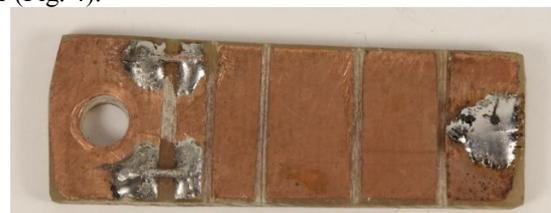
*Fig. 4. Surface breakdown plasma gun*
