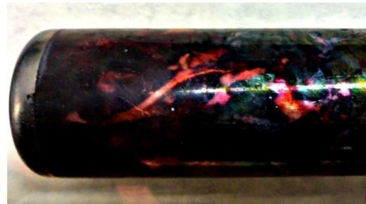
Fig. 7. Arc spot traces on the cathode
