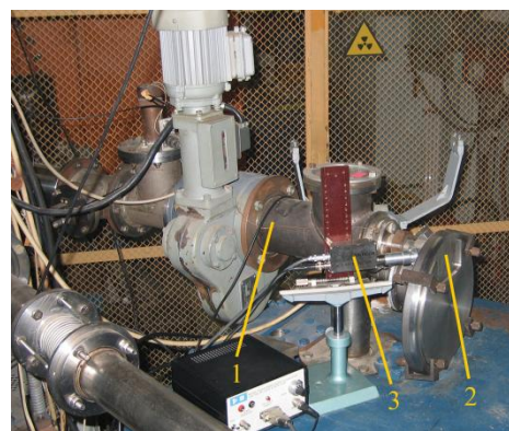
Fig. 1. Arrangement of the detectors relative to the proton beam and the target chamber: 1 – proton beam; 2 – target chamber; 3 – XR-100CR Si-PIN X-Ray detector
