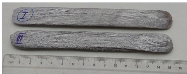
Fig. 2. External view of beryllium strips after extrusion at an angle of 90° to the applied load direction after deformation at 600°C (upper) and 500 °C (lower)
