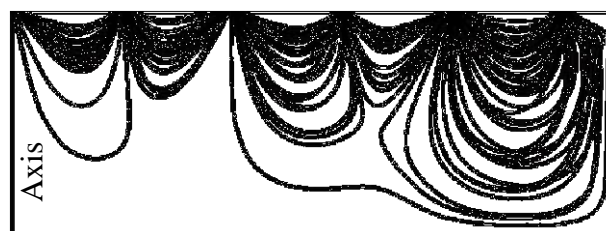
Fig. 4. Trajectories of particles in short chamber: a – top view; b – cross-section
