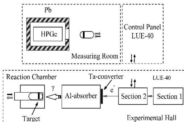
*Fig. 1. Experimental schematic diagram including three units shown with a dashed line. Above – the measuring room and the control panel of the LUE-40 accelerator, below – the experimental hall*
